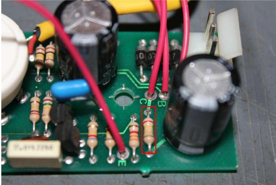
Replace R9 (red circle) with the 300k 1/2W resistor supplied with the kit.
