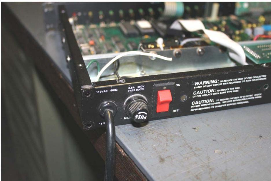
**Step 5:** Slide in the new kit, put the washers and nuts to the mounting screws and tighten it with a 5.5mm wrench.(Sorry, only metric nuts and bolts in the Netherlands,...) Put the two screws on the back of the corner back into their place and tighten them.
